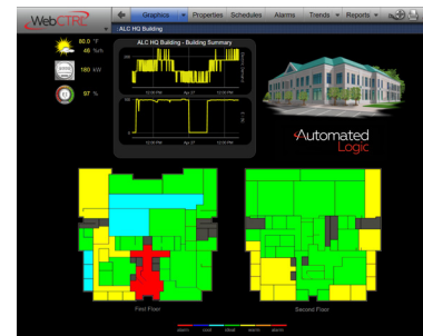
The WebCTRL building automation system is used to manage occupant comfort, water usage, and energy conservation measures.
