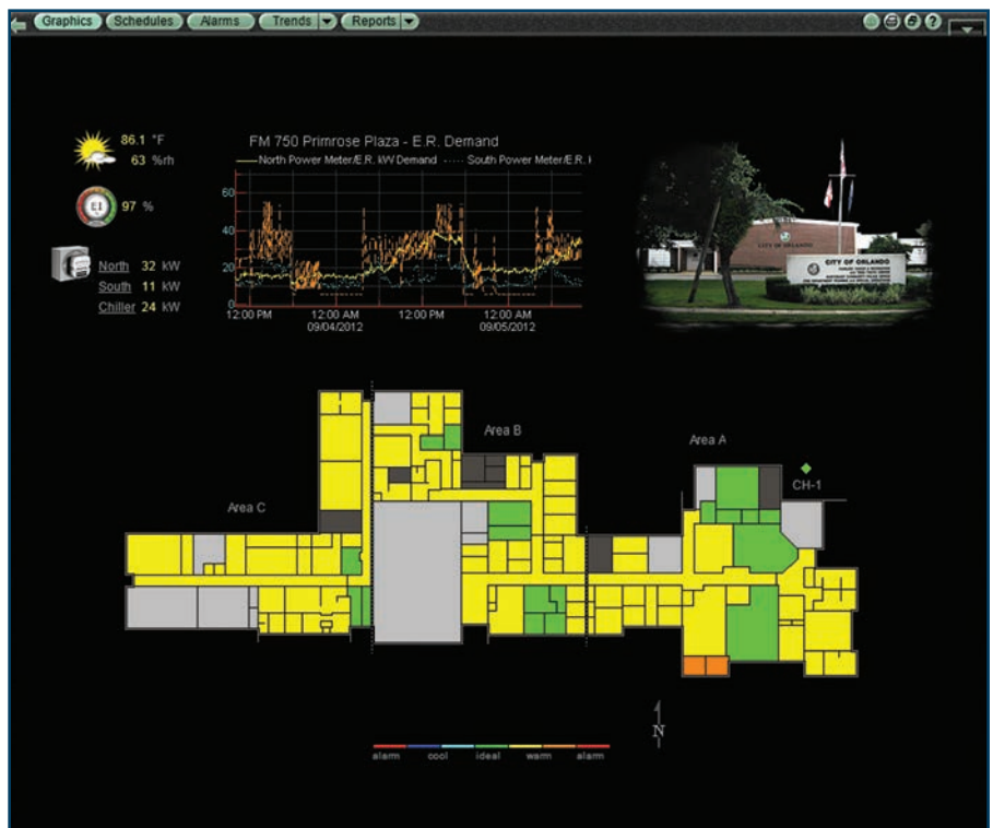
Figure 1: BAS summary graphic of Primrose Plaza, one of the larger buildings in this project. The gray areas indicate unoccupied rooms where sensors have turned off the HVAC to save energy.
