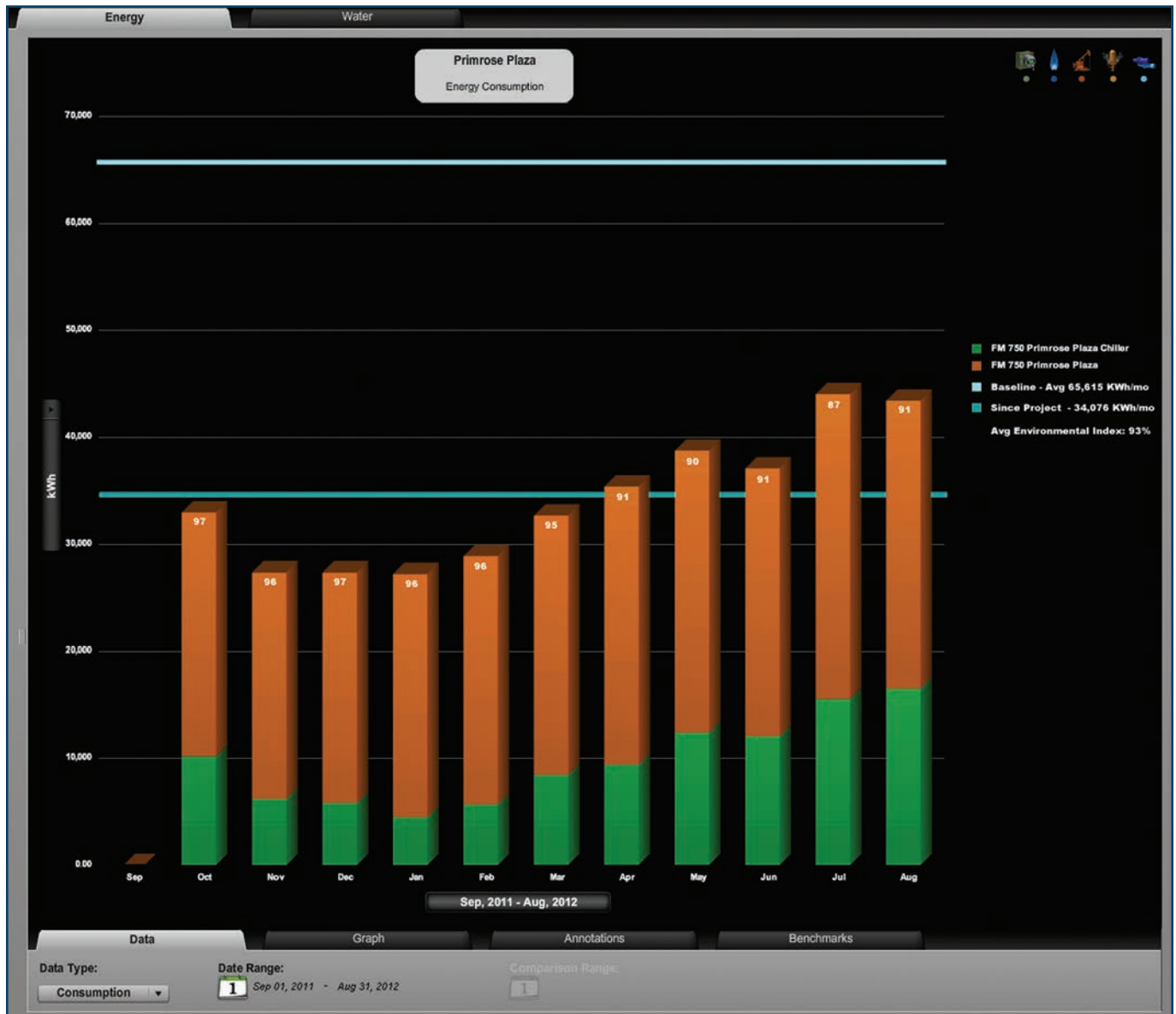
Figure 2: An energy reporting package screenshot of Primrose Plaza showing the energy savings resulting from a controls upgrade. The image has been annotated to include energy data from before the upgrade, as electronic metering was installed as part of the project. Occupant comfort is maintained even in the hottest months, as indicated by the average environmental index of 93%.
