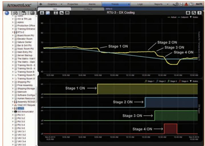
Figure 1: Temperature leaving the cooling coil (yellow line, top) drops when stages 1, 3, and 4 turn on, but there is no drop when stage 2 turns on.
