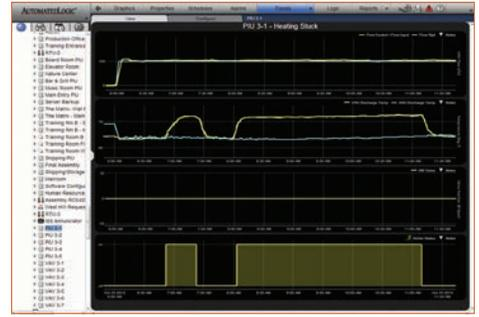
Figure 3: VAV box with heating valve not closing completely.
