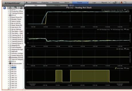
Figure 2: VAV Box reheat valve performance - normal.
