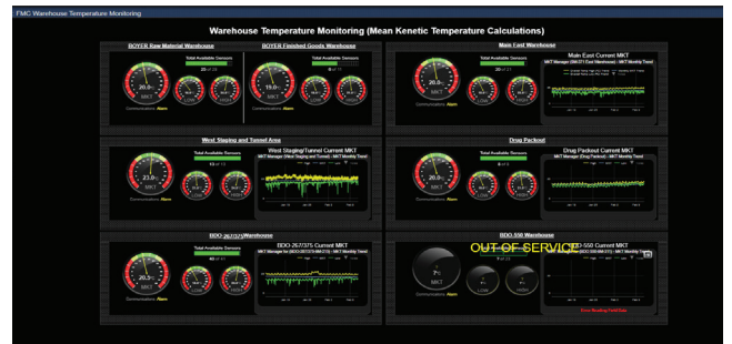
MKT compliance dashboard monitors environmental conditions across warehouse zones.
