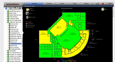
Thermographic color floor plans provide a snapshot of the building's operating conditions.
