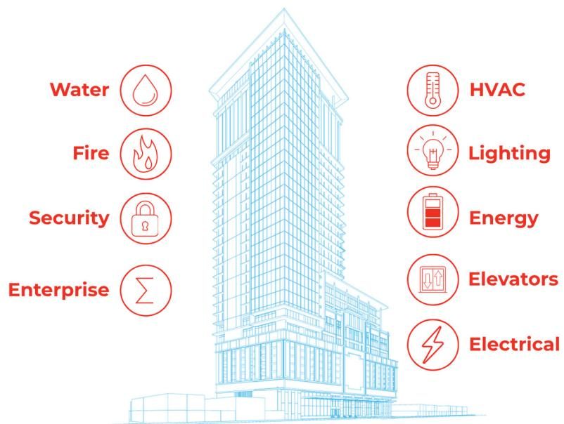
**Integration Scope Note:** WebCTRL® provides bi-directional control for mechanical (e.g., HVAC) and electrical systems. For Life Safety and Security systems (e.g., Fire, Access Control), the primary function is real-time monitoring and alarming for compliance, diagnostic, and reporting purposes.
